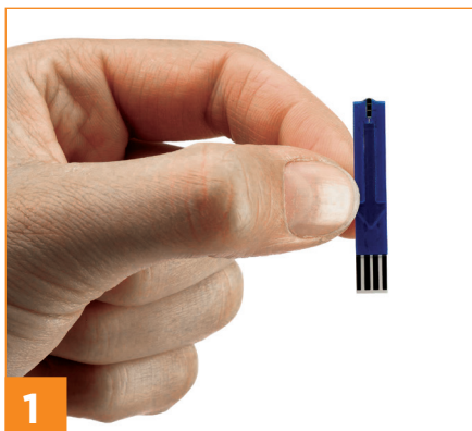
1 Remove sensor and place into analyser.
