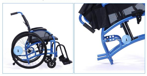
The further back the axle mounts are installed, the less likely the wheelchair is to tip over in use, i.e. in this configuration there is the least likelihood of the wheelchair tipping backwards. The further forward the axle mounts are installed, the lower the proportion of the total weight that is over the forward casters, making it easier to deliberately tip the wheelchair backwards (either by the user or the companion), which in turn makes the chair easier to maneuver.
