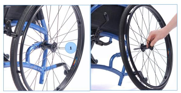
Press the locking button to attach the axle to its mounting. Release the locking button to fix the axle in place. Ensure that the locking button springs back into its initial position.
