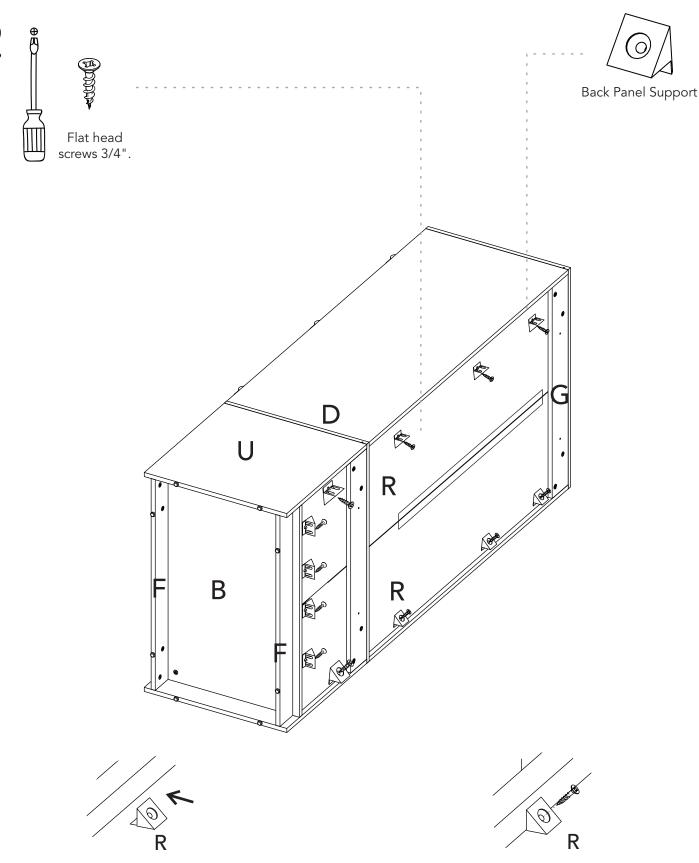
Insert the back panel supports between the gove and the back panel.
