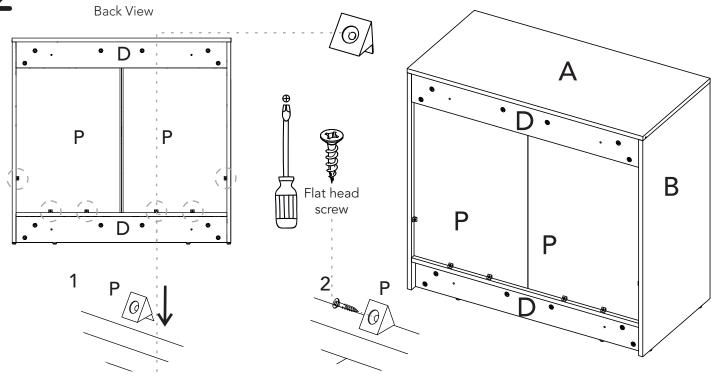
Insert the back panel supports between the gove and the back panel.
