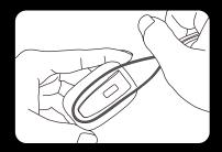
Loop lanyard in between the back shell and the clip.
