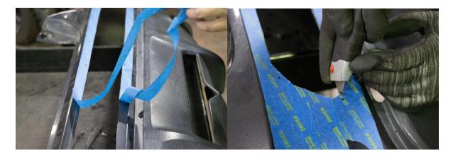
6) Place the Bumper Vent on the outside and the Backing Ring on the inside. Rivet together with existing holes first then from the inside out drill and rivet the rest of the holes.
