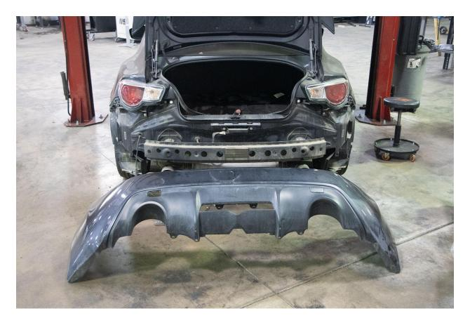
2) Mask installation area and mark center of bumper cover, use factory tow mount cover holes as reference.
