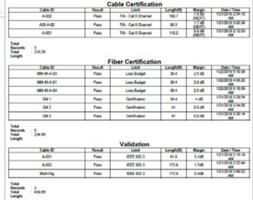
TestDataPro supports both PC and cloud-based options, and come standard with all models of TestPro. Printed test reports for copper and fiber optic include a listed of compliant network support based on the performance of the cable tested. Printed reports are provided for Copper & Fiber certification as well as the combined Multi-Gigabit/PoE Autotest. The Multi-Gigabit/PoE Autotest is a path to a new service offering you can provide to increase your revenue potential.
