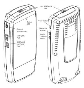
The AirCheck G3 is is a comprehensive, hand-held tool tool for network professionals to test and troubleshoot the latest wireless networks. The AirCheck G3 operates on 802.11a/b/g/n/ac/ax networks in the 2.4GHz, 5GHz, and 6GHz bands.
