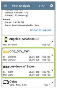
The AirCheck G3 is able to identify these Layer 2 switches and their interfaces because it has configured SNMP access to the switches.
