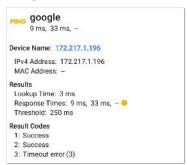
The third Response Time displays two dashes -to indicate that no response was received, and under the Results heading, the yellow dot points out the third Response Time as the reason for the Warning. Additionally, the third Result Code lists "Timeout error" as the reason for the Warning.
