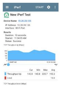
Test characteristics and status are displayed at the top of the iPerf results screen while the lower part of the screen displays a real-time graph of the TCP or UDP Upload and/or Download speeds. To pan and zoom on the graphs, you can swipe, double tap, and move the slider. See the Trending Graphs topic for an overview of the graph controls.
