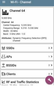
The Channel Details screen above shows how many SSIDs, APs, BSSIDs, or Clients are detected on Channel 64. Tap the lower cards in Wi-Fi Details to open a list screen that is filtered for the network component you are examining.
