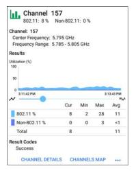
The Channel Test results screen indicates the **Center Frequency** and **Frequency Range** of the connected channel along with a real-time Utilization graph.
