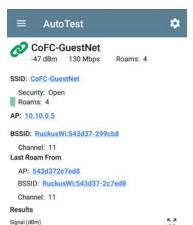
The Wi-Fi Link test screen shows these results:
