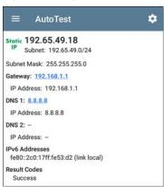
The Static IP test screen displays the configured addresses.
