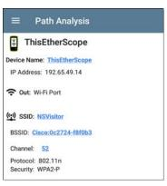
The example image above shows the SSID, Channel, and other Wi-Fi information the AirCheck G3 can display after running a Path Analysis over Wi-Fi.
