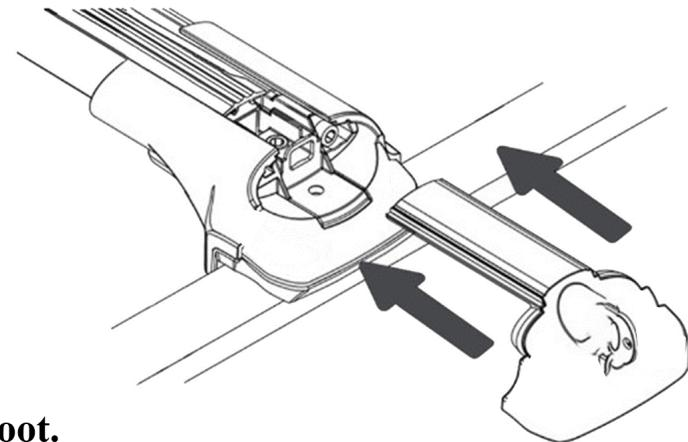
**Ensure each Foot is mounted correctly on the roof rail and each Metal Braket is alligned correctly bottom of the rail.**
