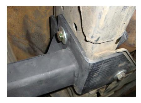
The (2)  $1 \frac{1}{2} x \frac{1}{2}$  bolts go in the lower holes on each side.
