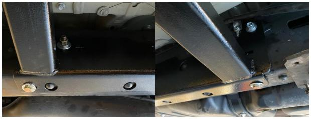
Rear most frame bolt is the 10MM bolt supplied. Reinstall the brake line over the slider mount. Install the Captured Bolt on the front frame hole Install the 3/8" bolts through the bottom of the frame.
