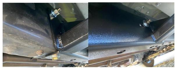
Passenger side rear mount: Two ½ Capture Bolts from inside of Frame through the slider, then fender washer, lock washer and Nut One 3/8'" bolt through the hole in the bottom of the frame with washers and nuts.
