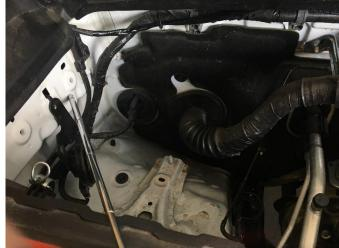
2. Place the first smaller Hefty Fabworks bracket into the side of the fender using two supplied 6mm bolts (C). Leave bolts slightly loose.
