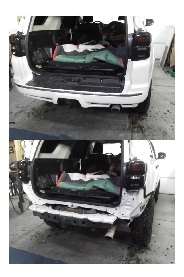
Once the Bumper cover is removed: Remove the hitch (saving the bolts) and the brackets on the under side of the frame. Remove the bracket that holds the trailer wiring but leave it hanging.
