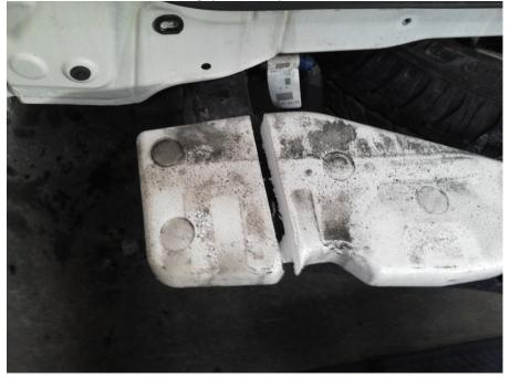
*Step 4:* Clearance. On each side of the fender there is a bracket that hangs down to attach the factory bumper cover to. Simply bend this bracket up toward the inside of the truck.
