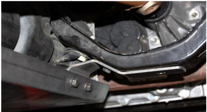
Secure the skid in place by adding the other M8 on the side of the skid driver side (LEAVE IT LOOSE) Install the last bracket – it works better if the rear driver tire is off – as shown in picture. Use M8's for the top and 3/8" for the bottom.
