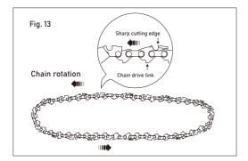
5. Starting at the tip, mount the chain drive links into the bar groove, leaving a loop at the back of the bar. The chain will loosely fit until it is placed on the sprocket (Fig. 14).
