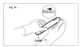
6. Hold the chain in position on the bar and place the loop around the sprocket. Fit the bar against the mounting surface so that the extruded piece on the mounting surface is in the long slot of the bar and the adjusting pin is in the chain tension pin hole (Fig. 15).
