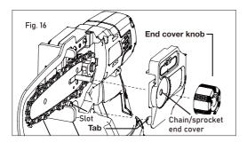
**NOTE:** Tool can't be operated when chain/sprocket end cover is removed; there is safety lock on the chain/sprocket end cover to avoid misoperation (Fig. 17).
