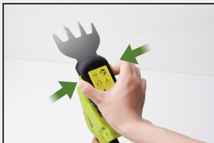
② Squeeze the lock button and remove the cutting head
