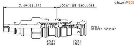
Pilot-operated, pressure reducing valves reduce a high primary pressure at the inlet (port 2) to a constant reduced pressure at port 1, allowing circuits with multiple pressure requirements to be operated using a single pump.
