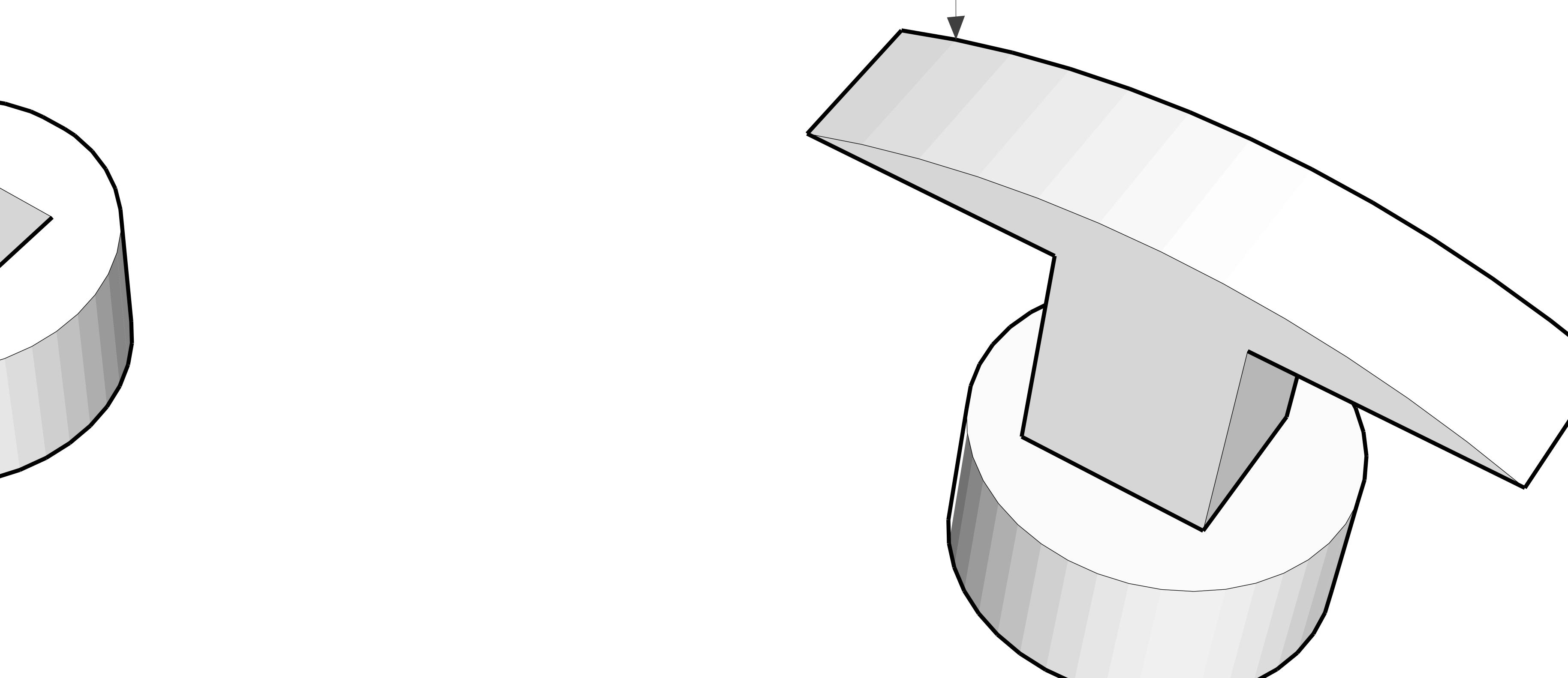
CAUTION: T-pins are fragile and can be extremely difficult to remove once seated.
