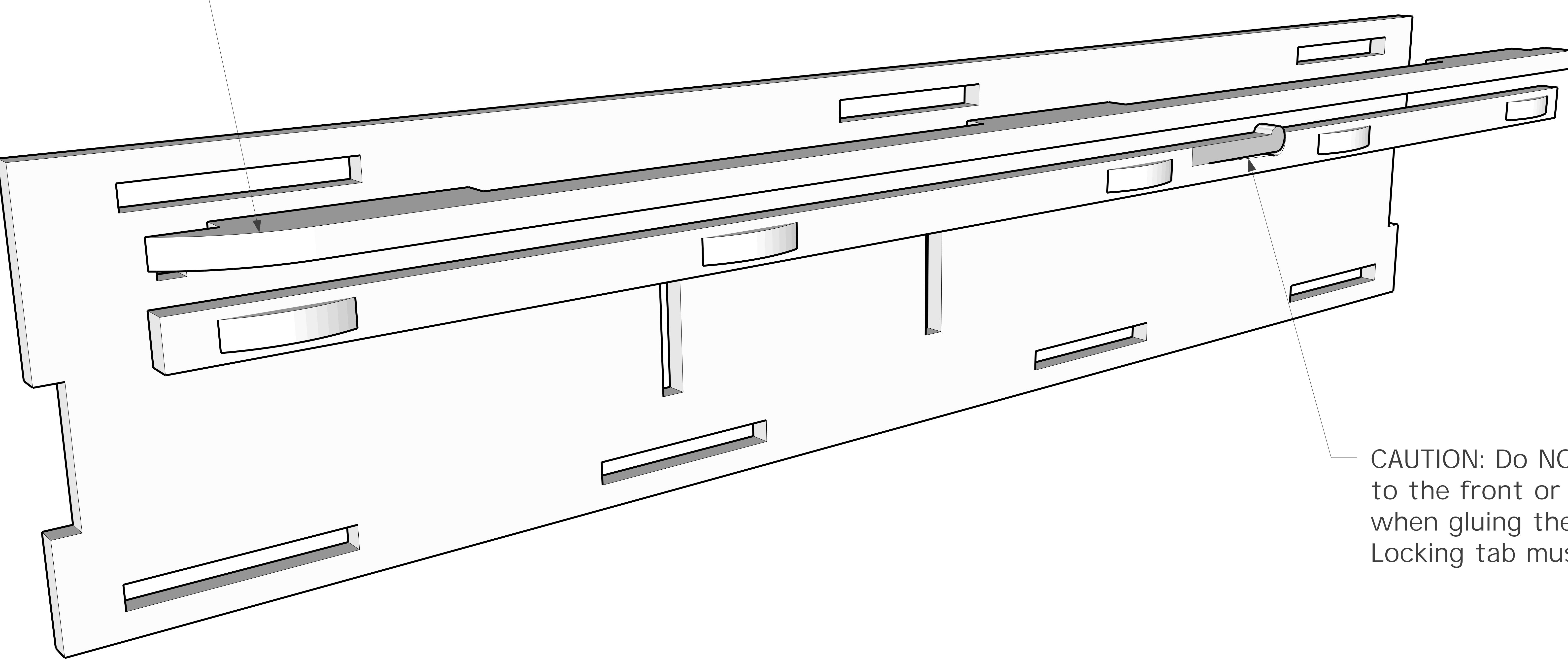
CAUTION: Do NOT apply adhesive to the front or back of the shade area when gluing the rail into position. Locking tab must be able to move freely.
