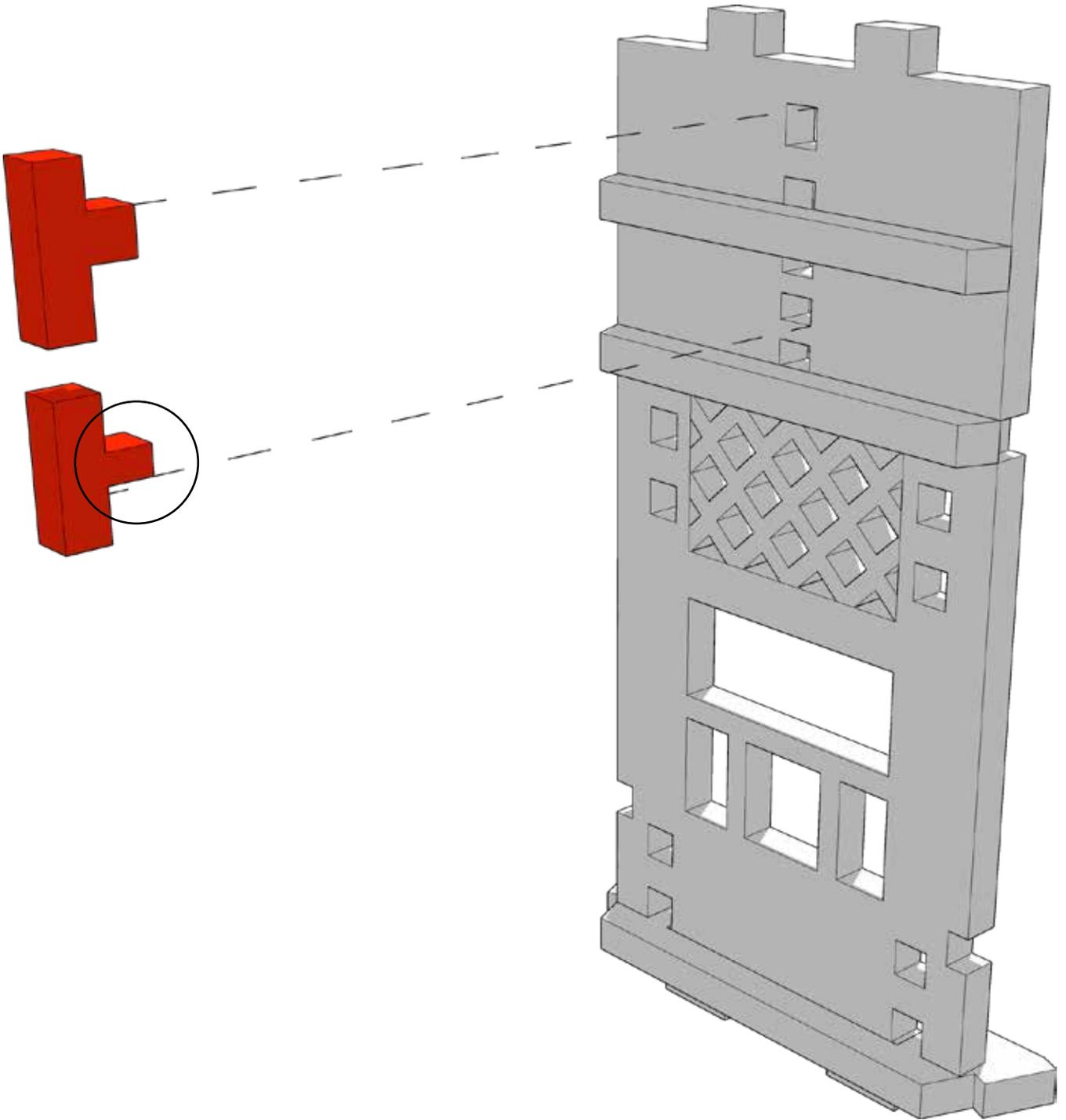
Circled part has a smaller tab than the one above and is labled "B" on the sprues. The other is labled "C"
