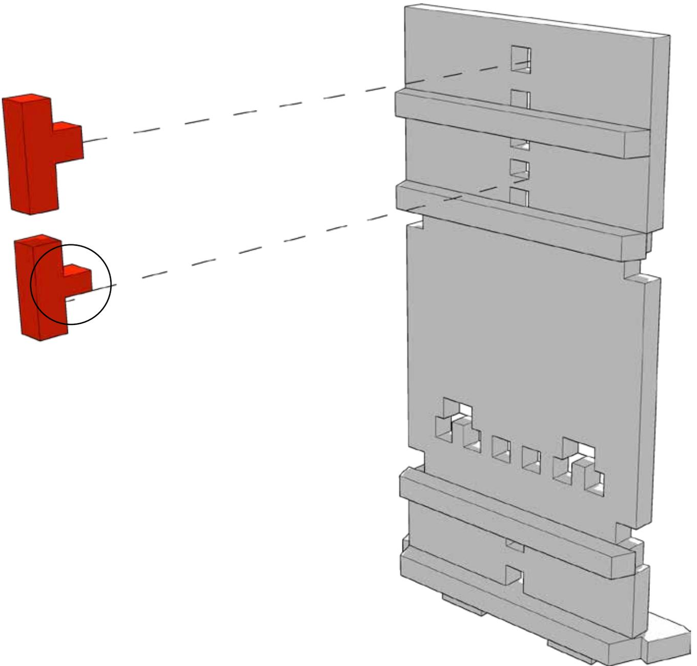
Circled part has a smaller tab than the one above and is labeled "B" on the sprues. The other is labeled "C"
