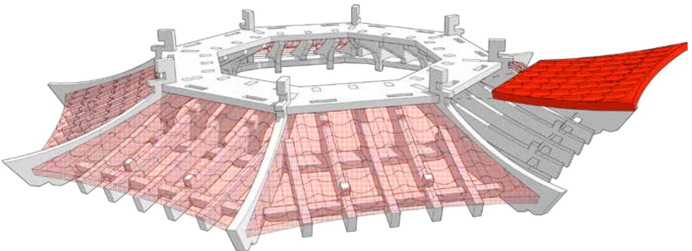
Roof sits under the larger hexagon part. Slot into place and align the tabs and push down. Using superglue or a fast drying glue is recommended. Repeat around the roof.
