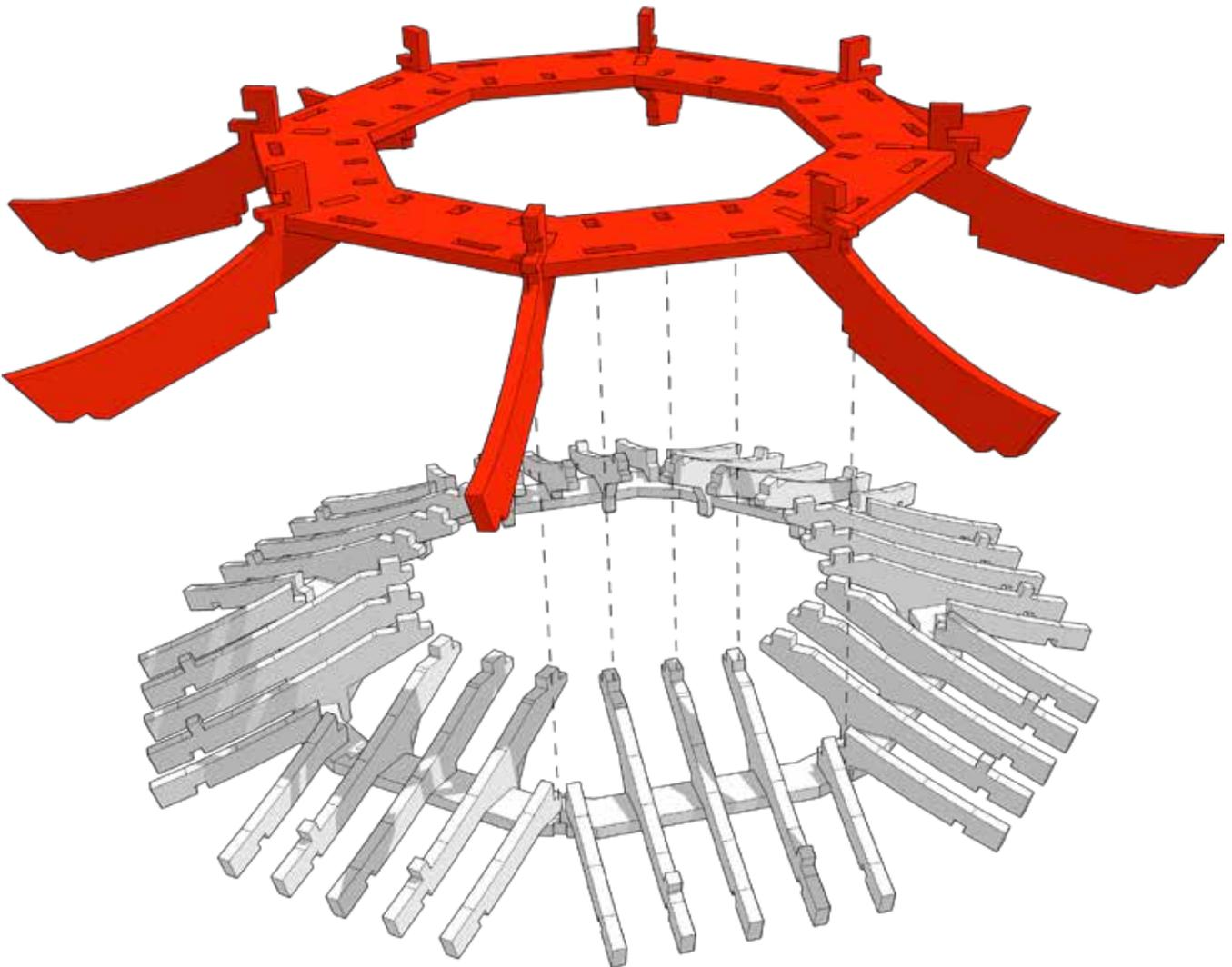
It is likely parts will pop out as you progressively slot this on. Be sure to check all parts are fully in place before glue dries.
