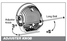
Adjuster Knob can be reversed from left hand to right hand side.
