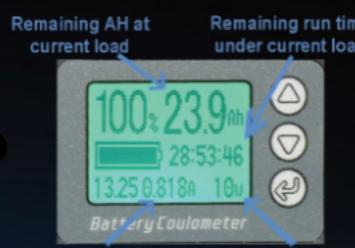
The screen will provide the remaining amp hour capacity, the current load in both amps and watts and the time remaining under the current load.
