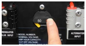
Only once the lower toggle on the isolation switch has been manually reset, will all of the connections within the Battery Hub be restored with power. If your Battery Hub is not operating, please check this isolation switch has not been triggered.
