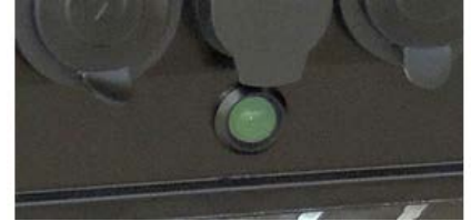
Figure 4 LED Indicator light Please refer to sticker on Thumper for current status
