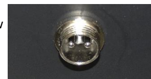
Image 3 2 pin Ignition activated feed
