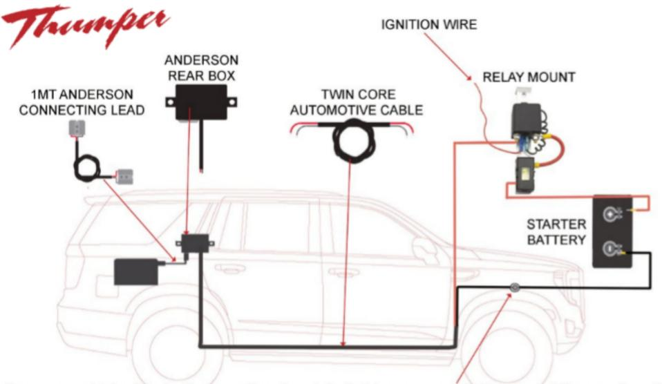
For newer vehicles fitted with a negative chassis bolt, it is recommended to connect the negative of the cable (6mm / 8mm) to this chassis bolt. All other vehicles will connect the negative cable directly to the negative terminal of the main start battery.
