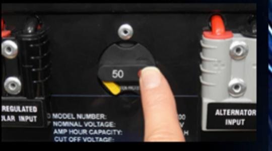
Note: The battery switch will be disconnected when originally purchased and must be reset before use.
