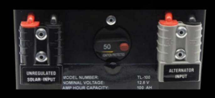
Vehicle charging must be connected via the Anderson labelled 'Alternator Input' in order to use the DC Battery Charger. If the DC charger is left to operate without an override, then the DC charger will engage its charge only when the vehicle's start battery reaches a voltage of approx. 13.2 volts.
