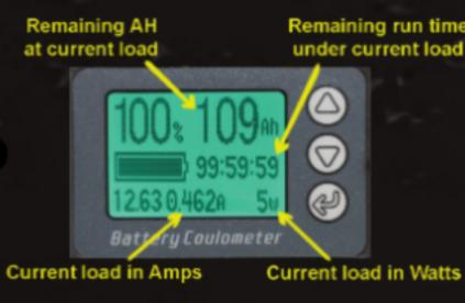
Remaining run time The screen will provide the remaining Amp Hour capacity, the current load in both Amps and Watts and the remaining run time under the current load.
