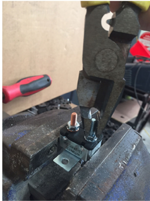
With a pair of pliers, grip one of the contacts of the circuit breaker and pull on it to remove it from its base
