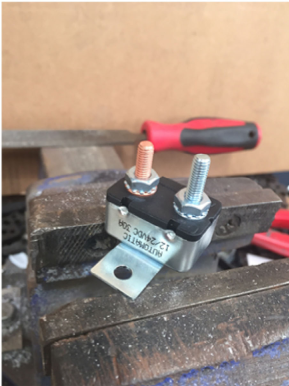
Circuit breaker (Prior to removing it from the metal base)
