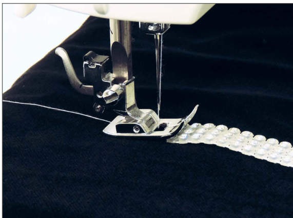
Inclined presser foot can cause problems with sewing machine feed of the base material.
