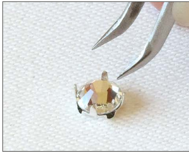
Manual bending and closing of the prongs with tweezers
