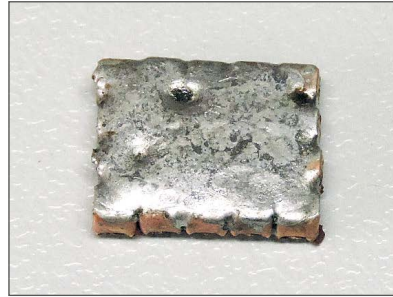
Solder applied on the whole product and heating of the whole surface
