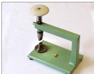
Device for prong closing when setting bigger stones
