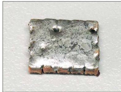
Too much solder (the solder flows over the cups)
