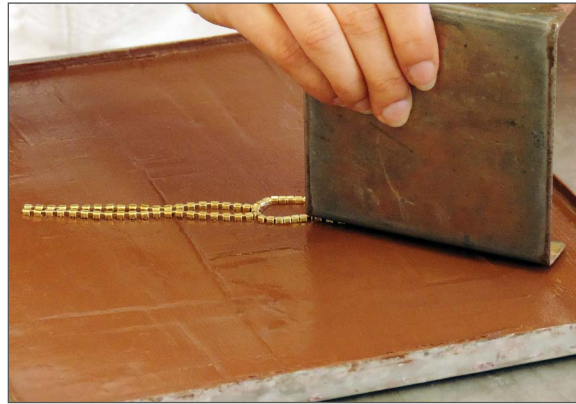
8 When the layout is definite press on the cup chain evenly using a small plate.
