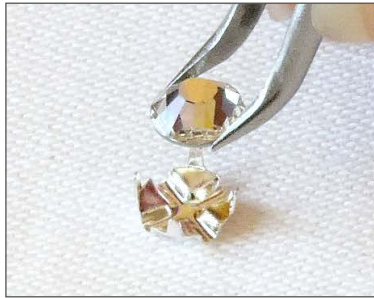
Setting the stone into the cup
