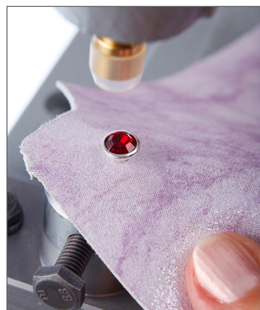
8. Applied Rivet from the top.
