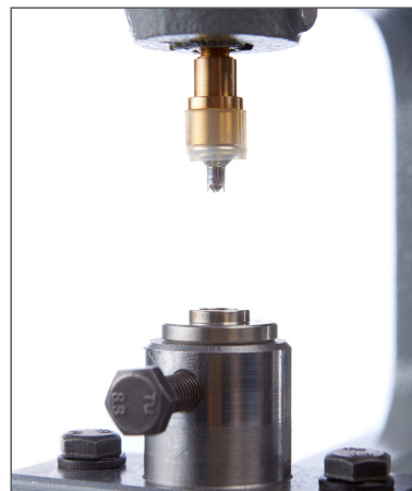
5. Attach the rivet to the upper die.
