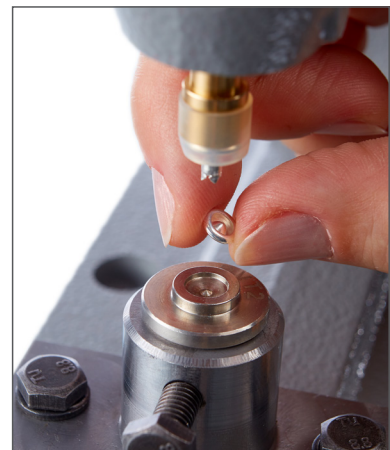
6. Place the back side of the Rivet on the lower die.
