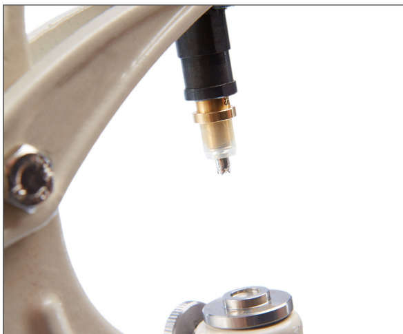
4. Attach the rivet to the upper die.
