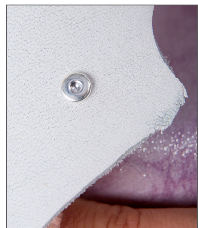
9. Applied Rivet from the bottom.
