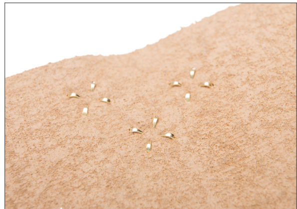
6. The application of rose pins from the bottom. The back side of the fabric should always look like this.
