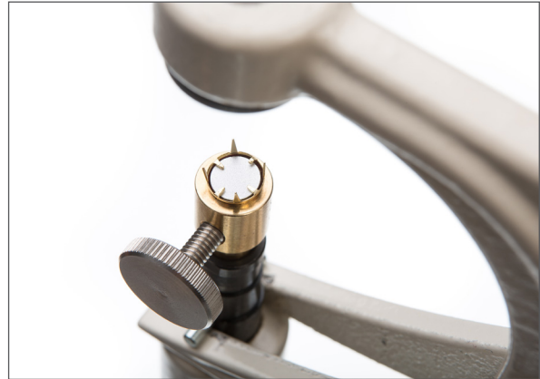
2. Put the pin into the upper die.
