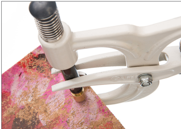
3. Place the fabric between the dies so that the rose pin is positioned where you want it. Make sure to punch it to the right side of the fabric. Squeeze the handles of the applicator.
