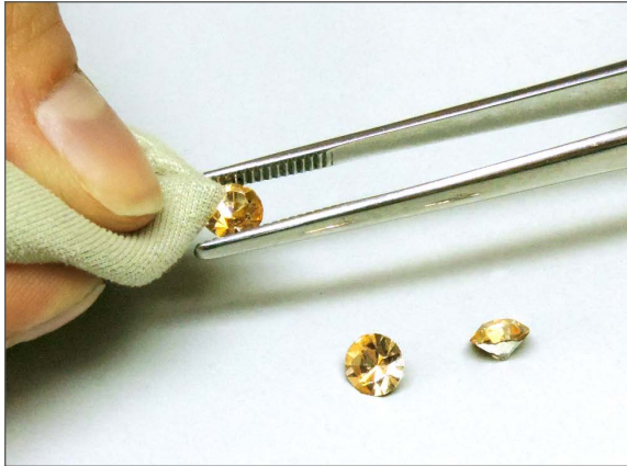
1 Clean the stones carefully before application (a cloth wetted in alcohol can be also used).
