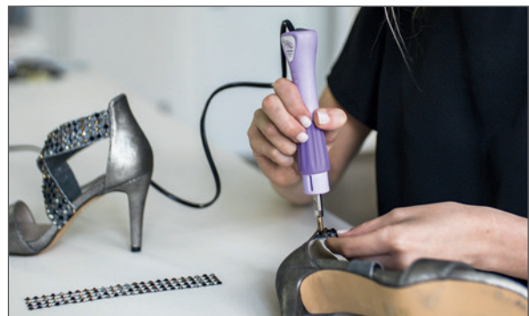
4. It is recommended to use the application head one size smaller than that of the stone being applied so as not to burn the string or the textile.
