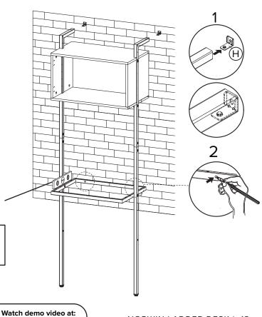
Make a hole in the wall on the pencil mark from previous Step 13.
