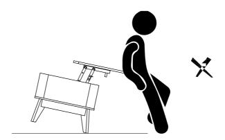
Please do not place any object on the table top while lifting, lowering, or moving the table.
