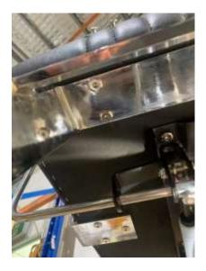
Remove the screws from the sides of the footrest, sit in place and replace the screws. Again, start them all first, ensure it is straight and tighten.
