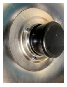
Lay the top of the hydraulic on a firm surface and tap the locator pin into the top of the hydraulic.
