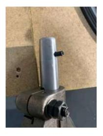
Put the plastic cover over the pump and inset the screw into the top.
