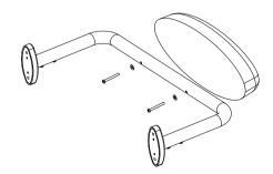
5. Tighten the backrest onto rail by washer and screws.
