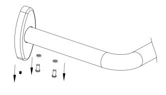
9. Backrest can be removed, if you want. Loosen screws on rails and screws on cover plates. And take off rail and plates.
