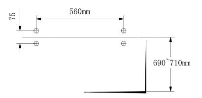
1. Before beginning installation, ensure that the wall is suitable for installing the backrest. Place the wall fixing plate on the wall at the correct height over the center of a stud and mark hole positions on the wall (refer to above picture). Tip: The backrest should be installed at a height of 690-710mm above ground level.
