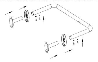
4. Slide the cover plate onto the rail, followed by inserting the wall fixing plate into the rail and securing it with a washer and grub screw.
