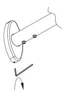
7. Reposition the cover plates onto the wall fixing plate and secure them by tightening the grub screw with an Allen key.
