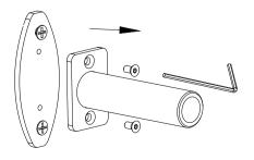
10. Loosen the screws on brackets (refer to above picture). Then you can take off the backrest.
