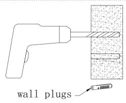
2. Drill pilot holes into the wall stud to a depth of approximately 60mm in order to accommodate mounting screws (and wall plugs if necessary). Tip: Use 3mm hole for screws into timber or 8mm hole for wall plugs.
