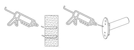
3. Reapply a small quantity of silicone to the wall fixing plate and the surrounding areas of the screw holes
