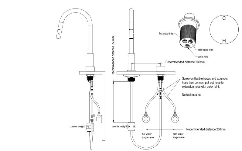
7. Turn the hand wheel counterclockwise to the end. Then reinstall the hand wheel, make the "C" should be on twelve o'clock direction and "H" on the six o'clock direction, according to above picture. Then tighten grub screw of hand wheel by allen key, put cap into hand wheel.
