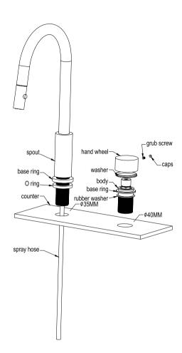
1.Drill a 35mm (for spout) and a 40mm (for mixer) through-hole on the counter.
