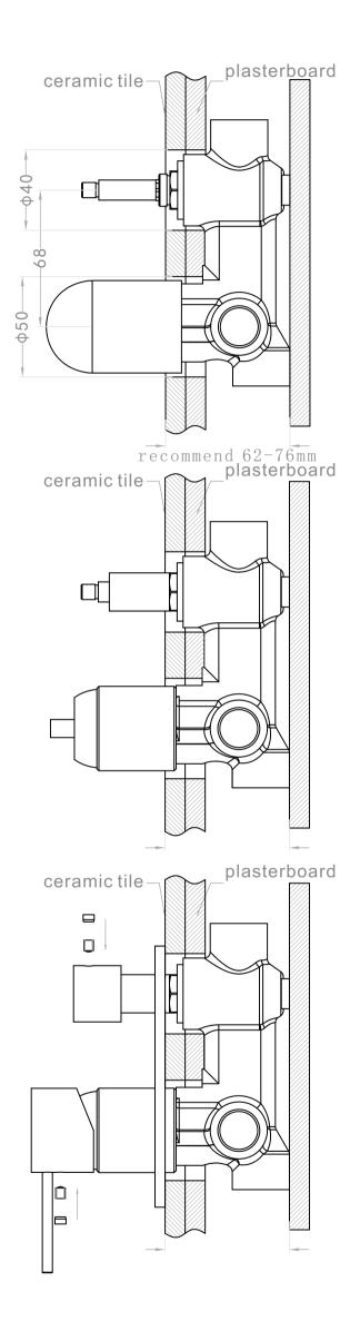
Fix body on noggin and ensure installation depth is 62-76mm from noggin to ceramic tile.
