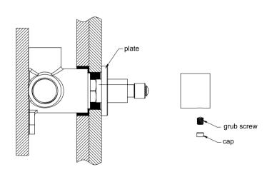
8. Put knob onto divertor cartridge, tighten it with grub screw using Allen key, and cap the grub screw hole.
