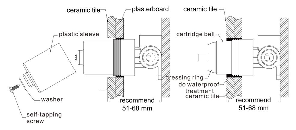
Drill a φ50 hole on ceramic tile, then install ceramic tile according to above picture.
