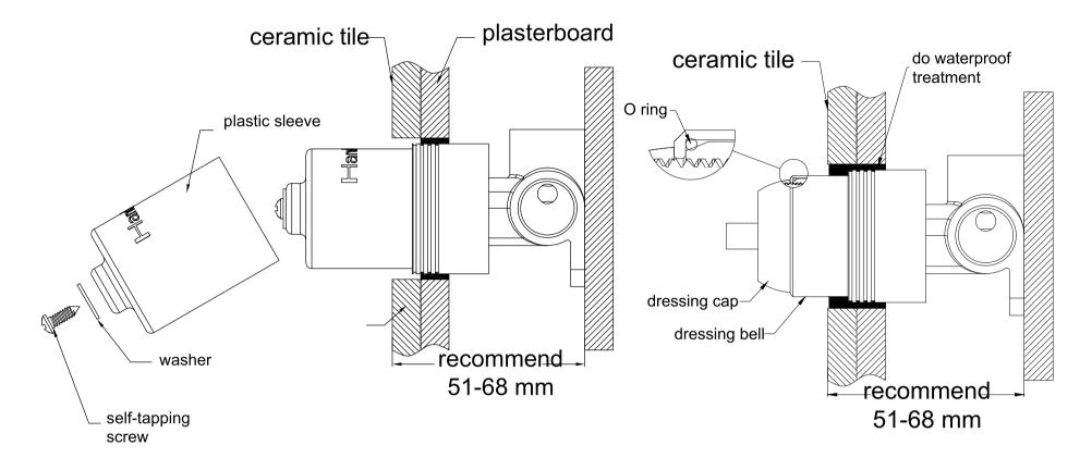
1.Drill a  $\phi$ 50mm hole in the ceramic tile, then position it as shown in the above diagram.
