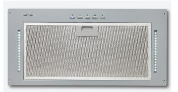
This unit comes standard with a charcoal filter mesh integrated with the aluminium filters for use in installations where it is used in recirculating mode. If the unit is installed in ducted mode the black charcoal foam sheet should be removed from the filter. The charcoal filters cannot be cleaned or recycled and must be replaced etc. Replacements are available from spares@eurolinx.com.au.
