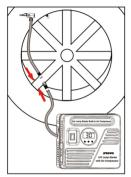
① Screw the extender to the hose attached to the unit.
