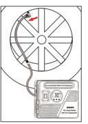
3 Press the lever down to clamp the hose to the tire valve stem.
