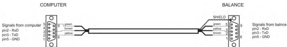
Scale – computer cable (RS232)
