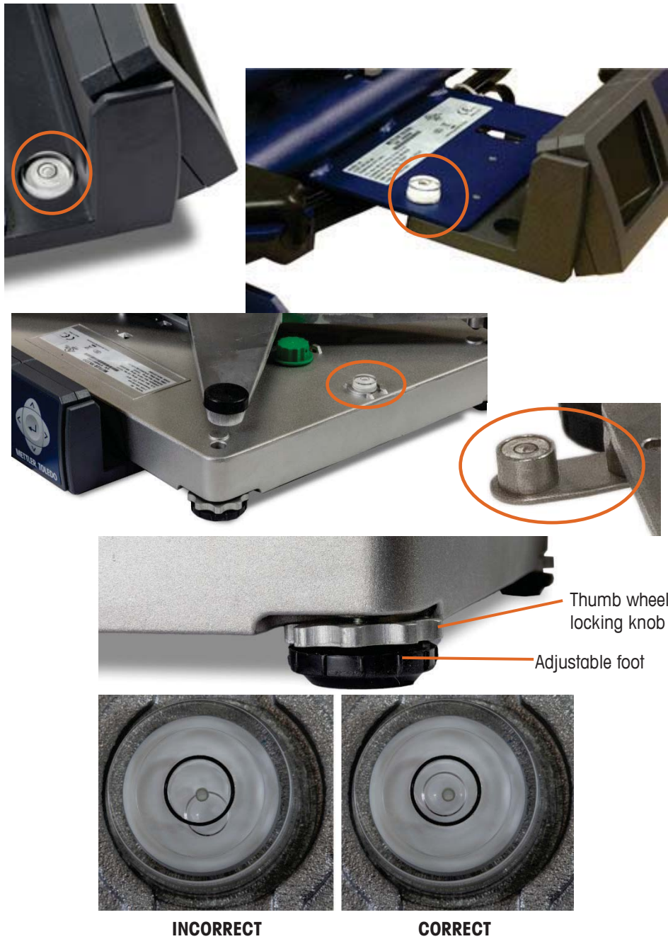
Figure 2-2: Leveling the Scale
