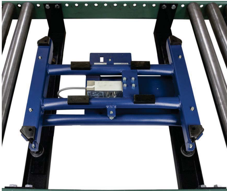
Figure 2-11: Conveyor Drop-In Kit Installed
