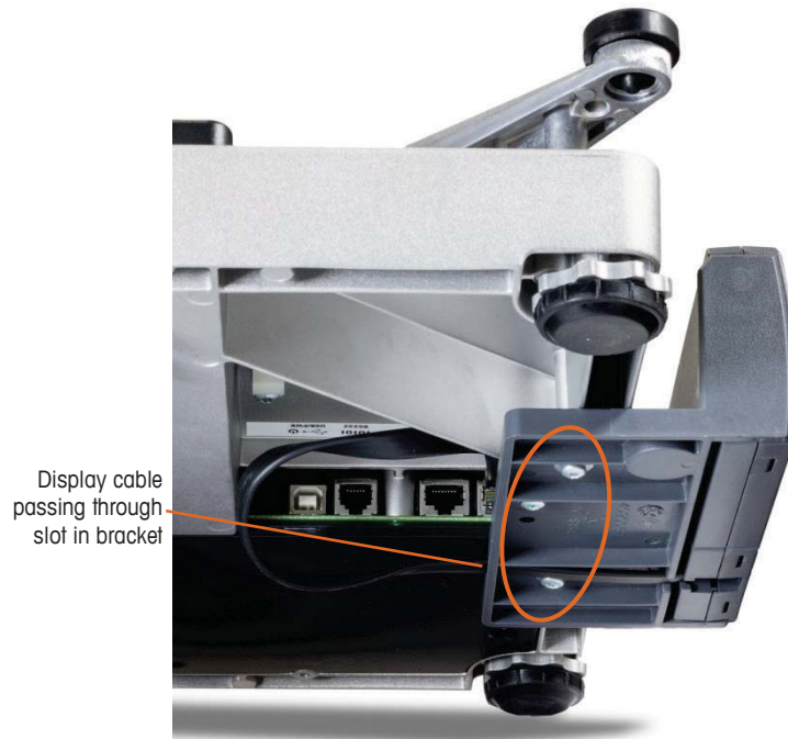
Figure 5-15: Display Mounting Bolts and Cable
