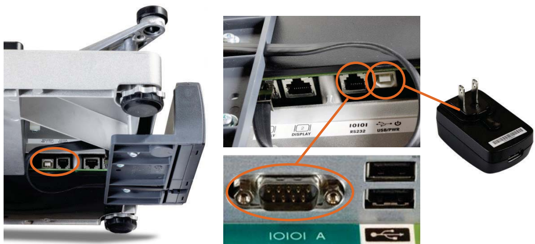
Figure 2-6: Serial Connections, Scale (left, top) and PC (bottom center); Power Supply (right)
