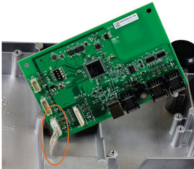
Figure 5-11: Load Cell Harness Connected to PCB
