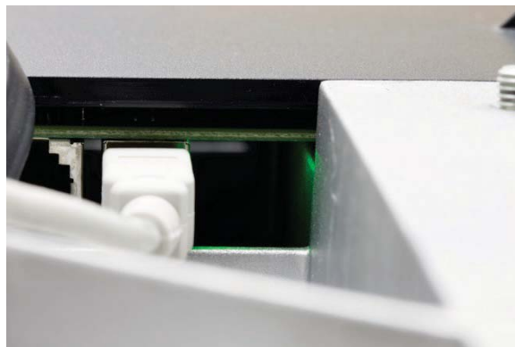
Figure 5-1: Green PCB Status Light Illuminated
