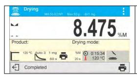
Upon drying process completion, summary of the test is displayed, final moisture content result is held, drying chamber's lid gets opened automatically. Upon process stop, printout footer is sent to a selected interface (accordingly to set printout options – parameter group DRYING PROCESS REPORT/FOOTER).
