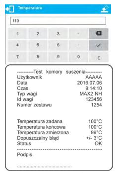
The temperature is maintained for 8 minutes (like for temperature adjustment procedure). After 8 minutes you shall see a window for entering temperature read from the installed adjustment set. Press button to confirm.
