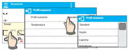
Enter drying profile settings and select respective drying profile. Upon selecting a profile, set its respective parameters. Parameters depend on selected profile.
