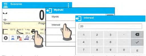
The time interval between printouts in seconds ranging from 0 to 120.
