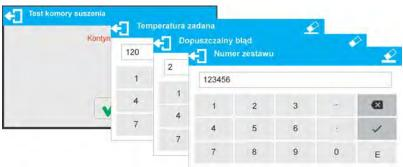
Enter testing temperature, maximum permissible error and the serial number of the temperature adjustment set.
