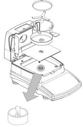
When installing the cross-shaped holder (pan supporter) pay special attention to the correct positioning of its mandrel. The mandrel features a cut providing unique positioning of the holder against the pan handle, thus preventing their contact and friction.
