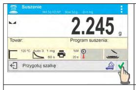
Press V button to zero the weighing pan weight.
