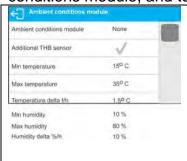
Ambient conditions module - parameter specifying module's working mode. Available options: **None** – readout of ambient condition module's indications turned off; **Record** – readout and record of indications into module's
