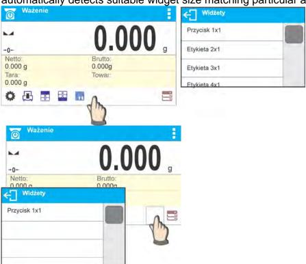
4. It is possible to change functions assigned to an already applied widget. The applied widget, if not needed, can be removed.
