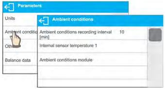
Ambient conditions recording interval [min]: parameter enabling you to specify record frequency of sensor-registered data, and to determine how often the displayed pictograms (providing information on ambient conditions state) are to be refreshed,
