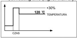
Specific feature of this drying profile is fast increase of drying temperature in short period of time. When compared to the preset temperature, the drying temperature rises 30% within 180 seconds and it is maintained at this level for a specified amount of time, next it drops to temperature value preset in drying profile parameters.
