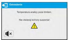
E. Follow the displayed prompt. Wait until the temperature decreases to a safe level, which is signalled by a new prompt.
