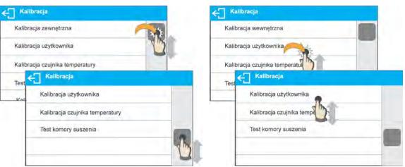
There are two methods for scrolling the screen of parameters window. The first one requires pressing, holding down and scrolling up or down the scrollbar located on the right. The second one requires pressing, holding down and scrolling up or down any point of the displayed window.
