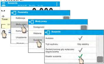
Enable the function to activate drying process wizard. The wizard guides you through all steps of setting the drying parameters. Only after setting confirmation the moisture analyzer will start the process of sample preparation and drying.
