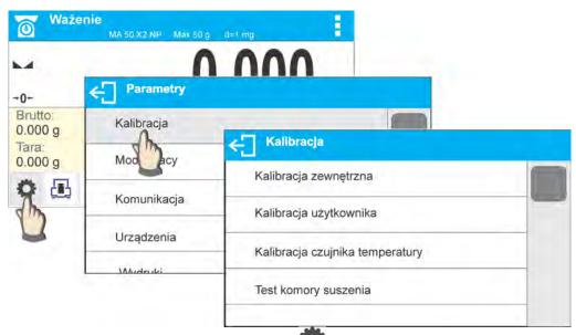
In order to enter moisture analyzer menu press <a>PARAMETERS> entry. Pressing any button comprised within workspace or pressing parameter name results with change of colour. If a given area has any function or action assigned, then it is performed automatically upon pressing (e.g. adjustment procedure), respectively a particular window with parameters or a list of appropriate settings is displayed.
